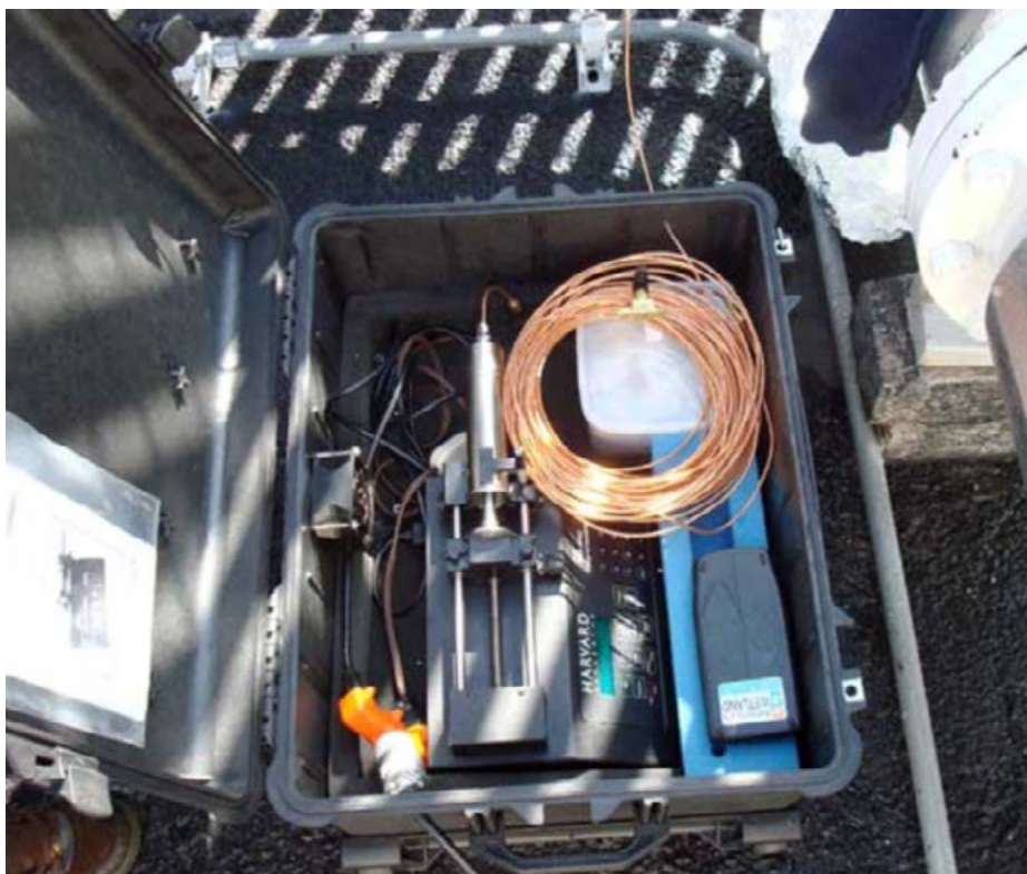
Figure 1 SPARTAH with all of its components: the Harvard syringe apparatus with syringe, Cu tubes, and power source inside a Pelican case. Picture from Barry et al. (2009)
