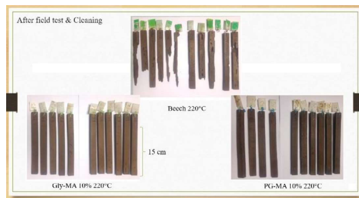
Figure 1 General principle of wood modification in the first section of the study (left) and appearances of certain modified woods after one-year duration of grave-yard test in a tropical country, Indonesia (right).
